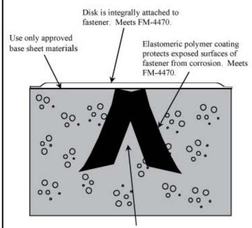
Fastener anchors itself in its own hole by cutting an inverted wedge of concrete. No pre-drilling required.
