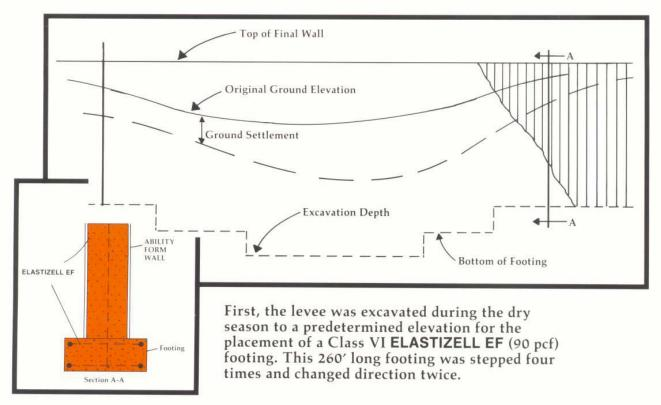
Next, to maintain the levee elevation for flood protection, a 12" wide ABILITY FORM WALL was anchored to the footing with reinforcing steel. The ABILITY FORM WALL cavity was filled with Class IV **ELASTIZELL EF** (42 pcf) providing an impermeable barrier against high water.
